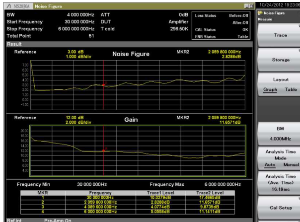
Measurement Result: Example of Graph display (Frequency Mode: Sweep, Screen Layout: Graph)
