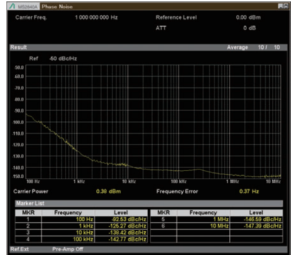
Phase Noise Measurement Low Phase Noise Performance MS2840A-066 On 1 GHz Measurement Frequency, Preamp Off
