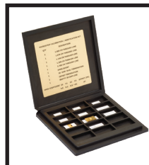
36804B-10M - 10 mil Microstrip Calibration/Verification kit
