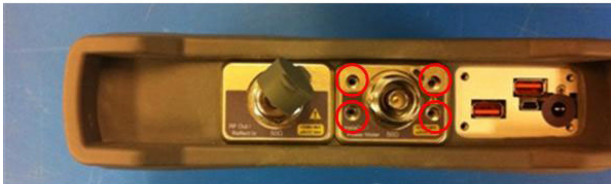
Figure 4-12. InstaCal / Power Meter Removal
