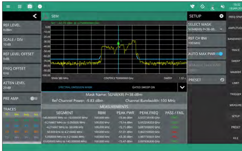
OTA SEM measurement on a 5G NR transmission with pass/fail results
