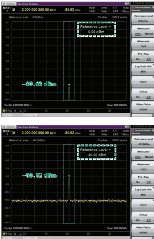
Example: Level Stability by Switching Reference Level
