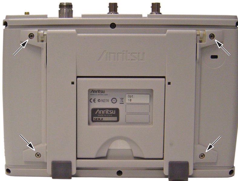
Figure 4-14. Remove the Four Screws to Replace the Tilt Bail
