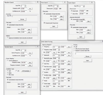
Discrete search engines are available for locating carrier, wireless standard, and arbitrary waveforms.
