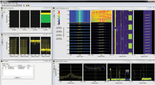
Simultaneously view and analyze up to four signal files (channels). The user can choose frequency, time, and magnitude plots for each channel.
