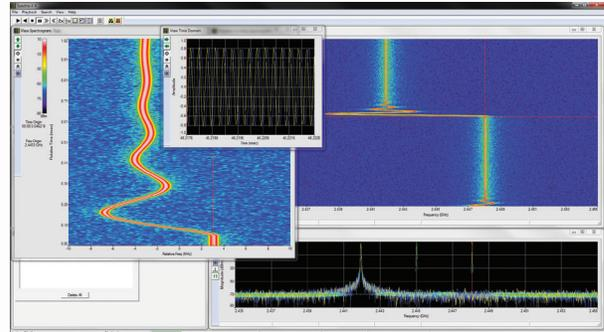
Spectrogram time windows positioned in time and frequency by marker placement. View Spectrogram and View Time-Domain Plots provide high-resolution, with finely detailed snapshots of transient events.
