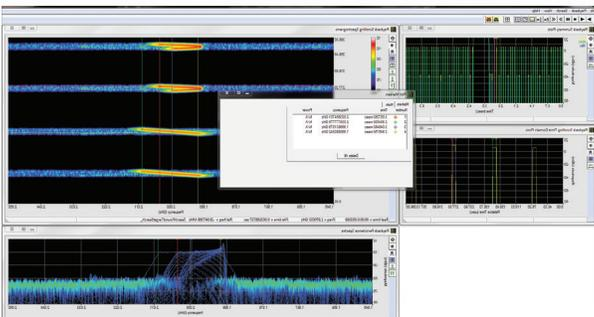
User-defined marker math allows time and frequency differences to be measured within or between channels.
