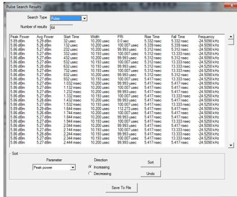
Pulsed waveforms can be searched for and characterized by their rise and fall times, pulse width, pulse repetition interval, peak or average power, or carrier frequency.
